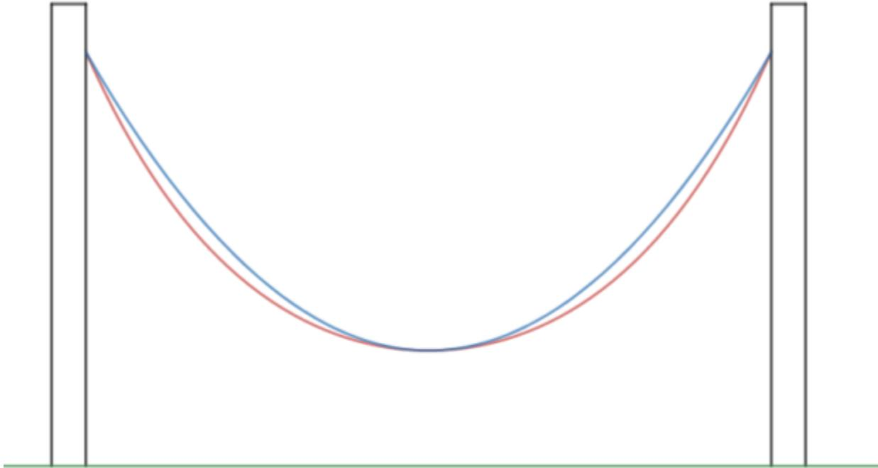
Fig 3. The catenary (in red) and the parabola (in blue) have very similar shapes, but they are different curves.
